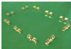
Shield-can clips reflow soldered onto PCB
